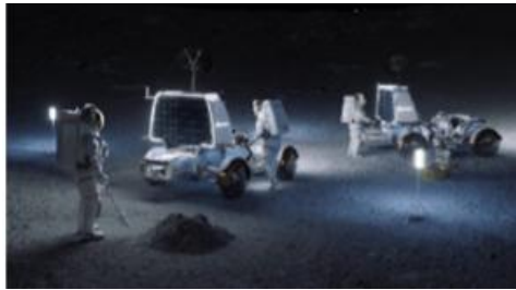
Figure 11: The Pegasus rover, designed to work in manual, autonomous and teleoperated modes for missions of up to a year. Photo: Lunar Outpost.
