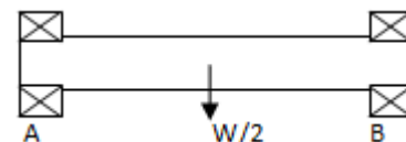
Figure 5: Load acting on idlers
