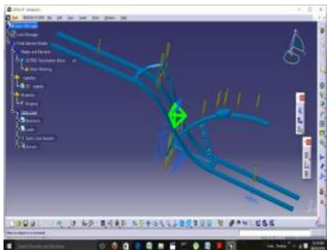
Figure E: Displacement pattern for aluminum chassis.
