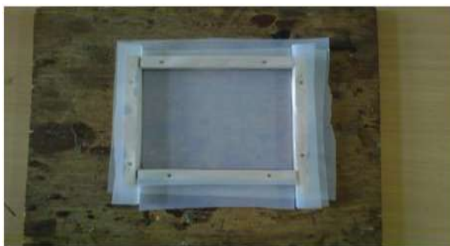
Figure 3.1: Mould used for fabrication of the composite
