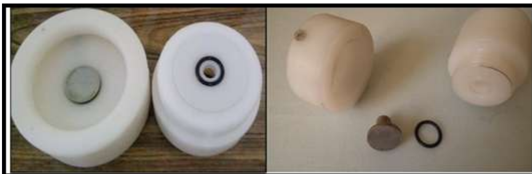
Figure 1: Show the parts of Teflon cell used in work
