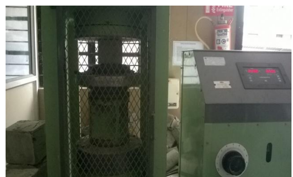
Figure 1: Concrete specimen subjected to compression
