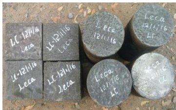
Figure 2: Cube and cylinder specimens
