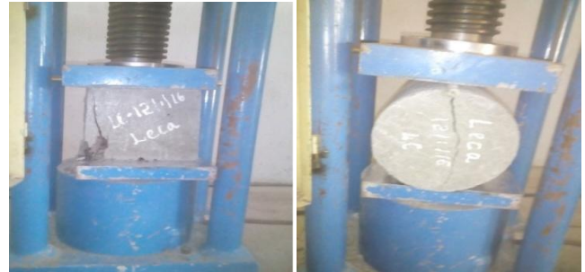
Figure 3: Testing of cube and cylinder specimens
