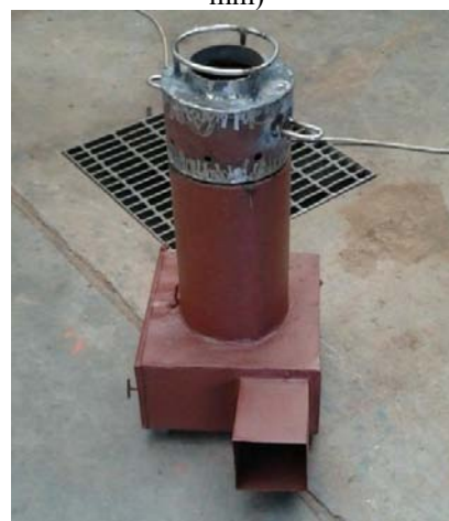
Plate 3.1: Gasifier stove under fabrication
