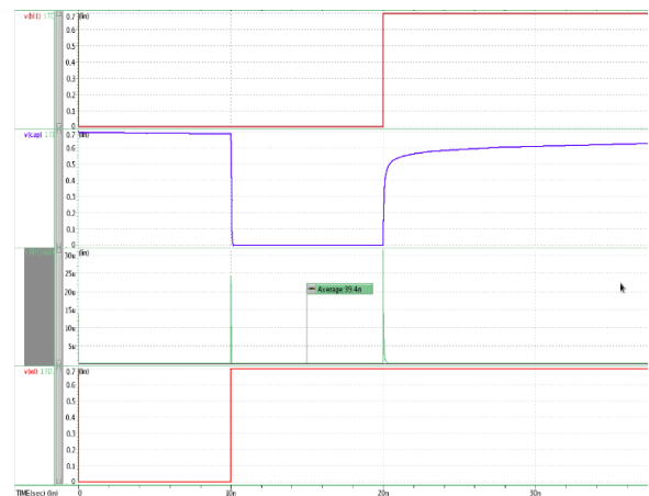
Figure 20: Read cycle of 1T1C DRAM cell
