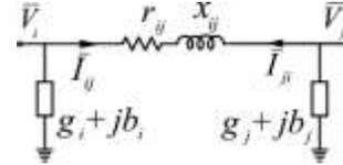
**Figure 1:** Two port  $\pi$ -model of transmission line
