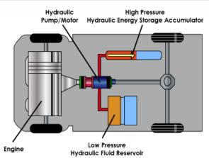
This figure demonstrates the inverse, the high pressure accumulator releasing energy during the acceleration process.
