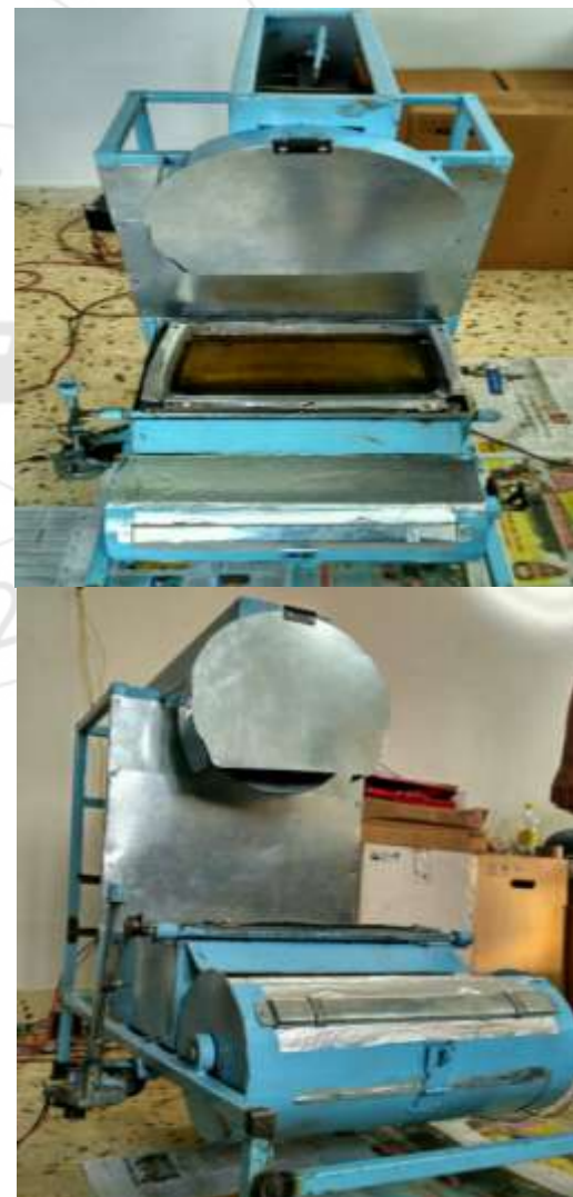
Figure 13: Prototype of Integrated potato chips making machine
