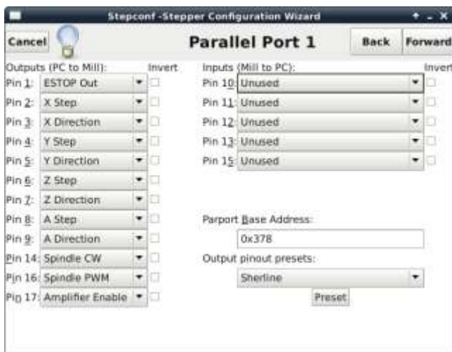
Figure 7: Stepconf setup page for 4 axis
