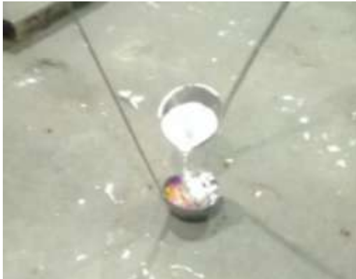
Figure 3: Molten Aluminum being poured
