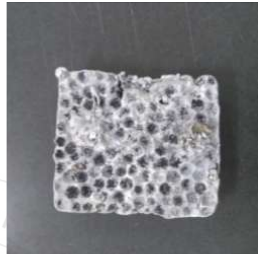
Figure 5: Thermocol bead cast
