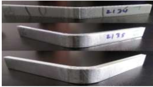
Figure 9: Bending sample after test
