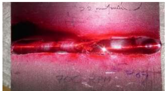
Figure 5: Penetrant is applied on weld surface
