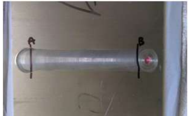
Figure 3: Top Surface of weld joint
