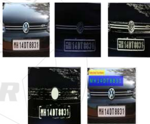
Figure 3: Processing of captured image to detect numbers of number plate
