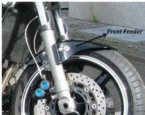
Figure 2: Mounting of proximity sensor – front fender
