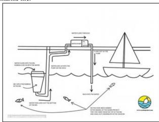
The Sea-Bin is capable of removing only solid wastes from the water it is placed in. With a device like that in place, the need to removed dissolved chemicals remains.
