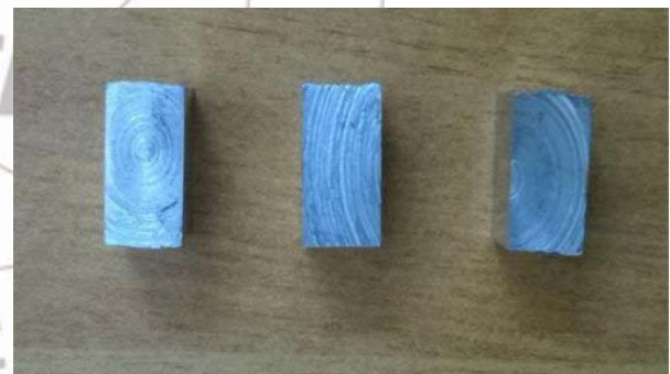
Figure 3.8: Density test specimens
