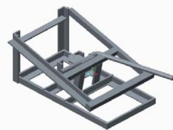
Figure 2: Isometric view of the coconut dehusking equipment.
