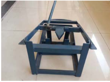
Figure 4: Pictorial view of the assembled coconut dehusking equipment.
