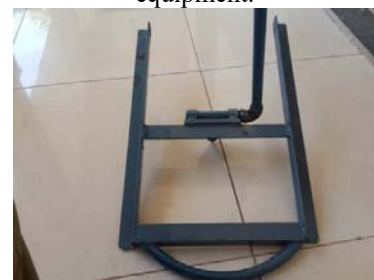
Figure 3: Pictorial view of the main frame of the coconut dehusking equipment.
