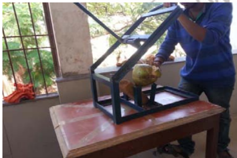
Figure 6: View of the coconut dehusking equipment during operation.
