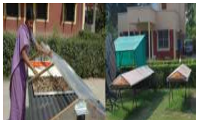
Figure 1: Solar dryer for vegetables
