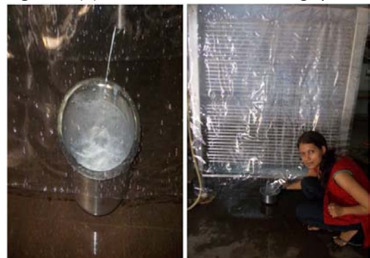
Figure 2: View of collection of hot milk from surface heat exchanger
