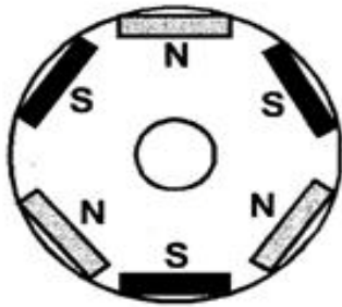
Figure1. Circular core with rectangular magnets embedded in the core.
