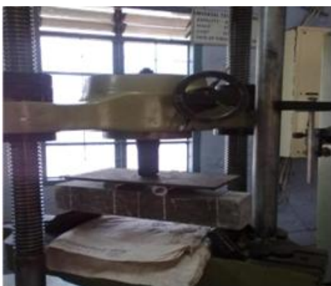
Figure 6: Flexural strength test set up
