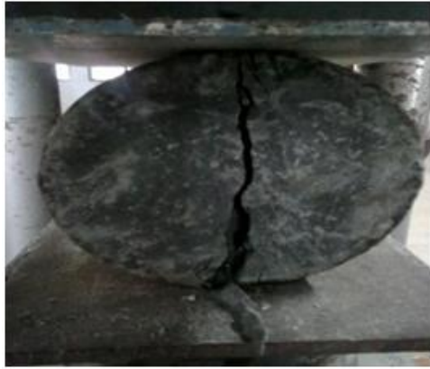
Figure 5: Split tensile test set up
