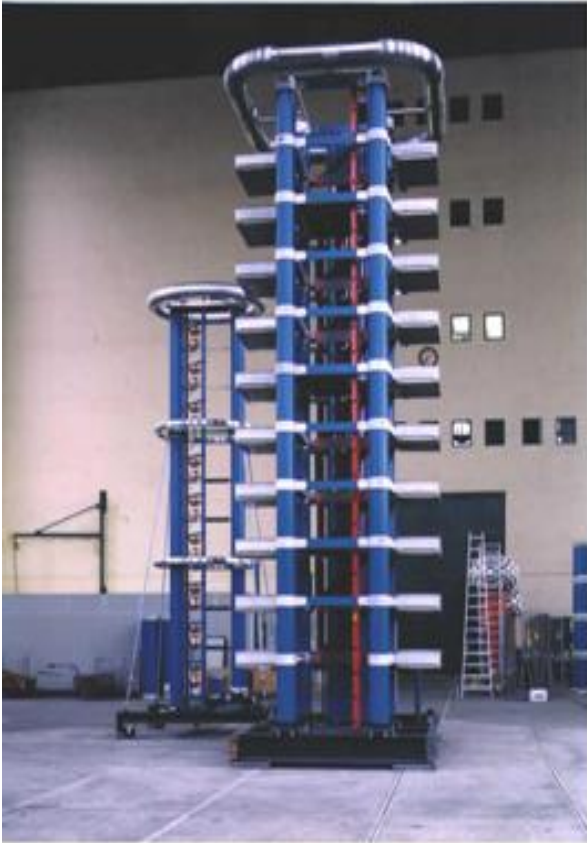
Figure 5: Impulse Voltage Test System IP 150/2000 G (150 kJ, 2000 kV) with impulse voltage divider and chopping multiple spark gap, with a stage energy of 15 kJ being used for the I test of power transformers up to 245 kV
