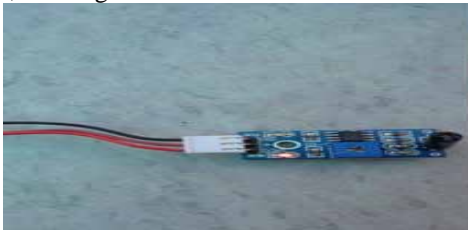
Figure 5: Snapshot of vibration sensor RF module
