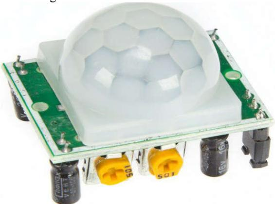
Fig 3.3 Motion sensor
