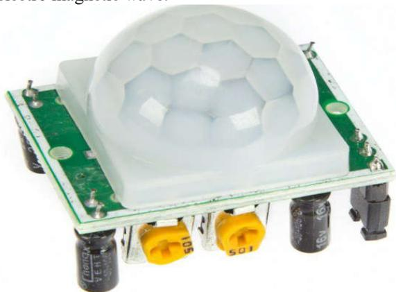
Fig 3.3 Motion sensor
