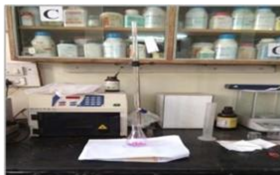
Figure 5: Measurement of IEC of Nafion™-117 Membrane
