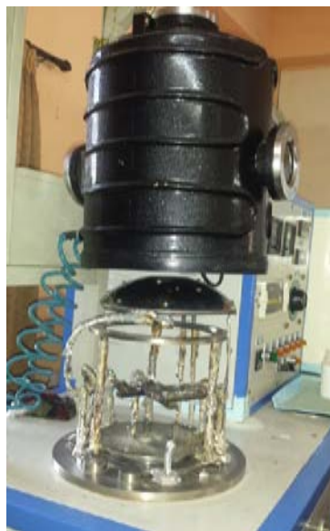
Figure 2: Thermal Evaporation Unit
