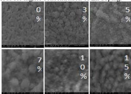
Figure 2: SEM images of pure and Zn doped CdO thin films (a) 0%, (b) 3% (c) 5% (d) 7% (e) 10% and (f) 15%
