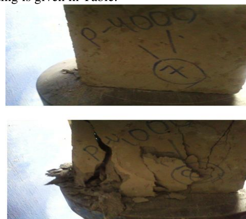
Figure 5.2.1: Application of load on cube and Compressive strength test on cube (PEG 4000)
