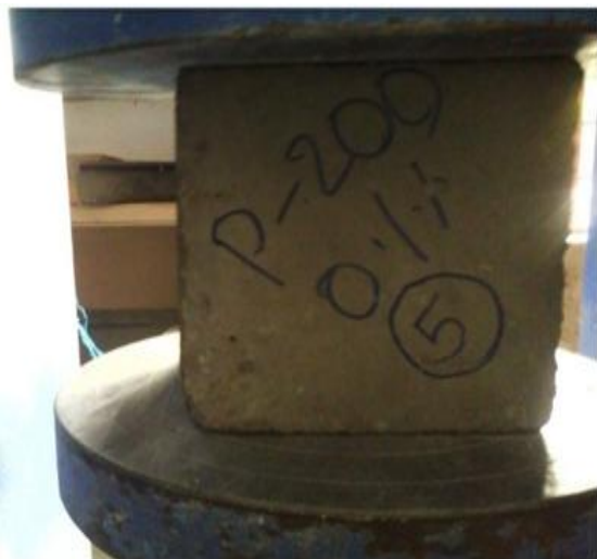
Figure 5.2.2: Application of load on cube and Compressive strength test on cube (PEG 200)z
