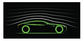
The flow of air in a certain manner according to the shapes it faces is called not aerodynamics rather the study of it. When a car is driven at high speeds it faces an opposite force called air drag. This air drag is detrimental to the fuel economy as it causes the engine to output more power to counter it. At a small time frame, it's not much but over a long time, it causes enough opposing force to make a dent into your fuel economy (pun intended).
