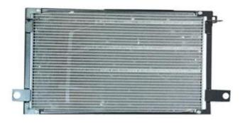
The job of the condenser is to convert the gas that AC compressor provided it into liquid. It does so with the help of an AC fan which blows cool air into the condenser. It is to be noted that the condenser does nothing to pressure state. The cooling, however, has an effect on the gas converting it into a liquid which is at a normal temperature.
