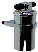
This step doesn't do anything to the refrigerant but to clean it. The Receiver dryer removes any contaminants from the system which can harm the system and cause it to fail. The liquid passes through after being cleaned. This contaminant is moisture and is cleaned by aproduct called a desiccant. It absorbs moisture if any present thus cleaning the refrigerant.
