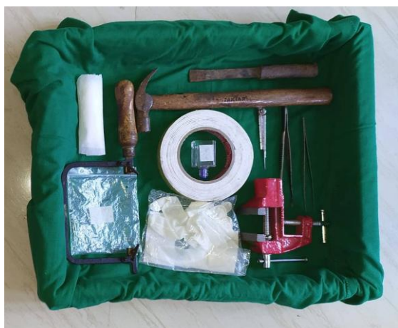
Figure1: Materials used for Jeweler’s cut (Jeweler’s Saw, Climax Fixed Base Table Baby Vice, Both Side Tape, Chisel, Hammer, Fine Forceps and Probe or Needle, Gloves, Gauge pieces and Marker pen)
