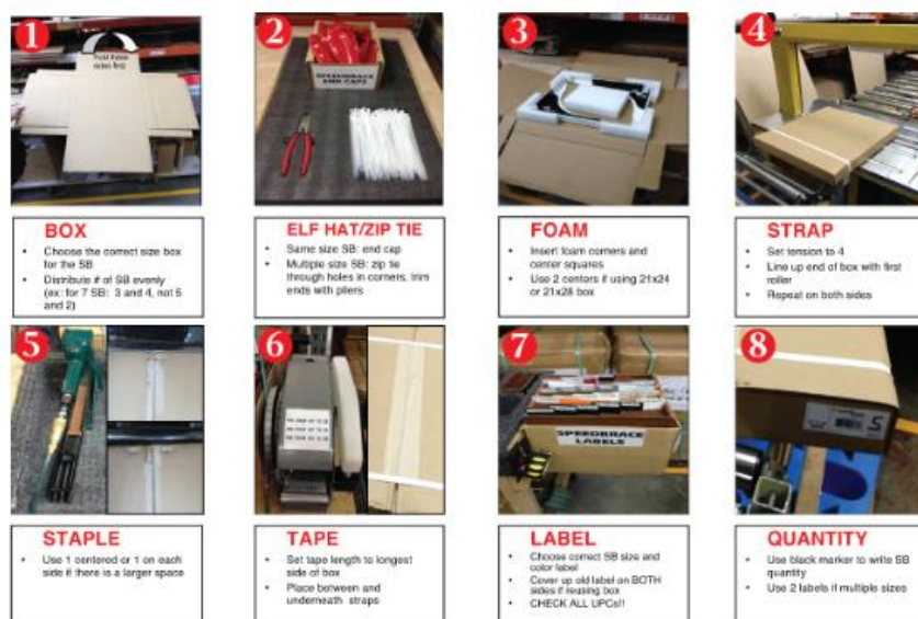
Figure 2: The standardized work instruction defines in detail all work elements performed by operator on assembly station
