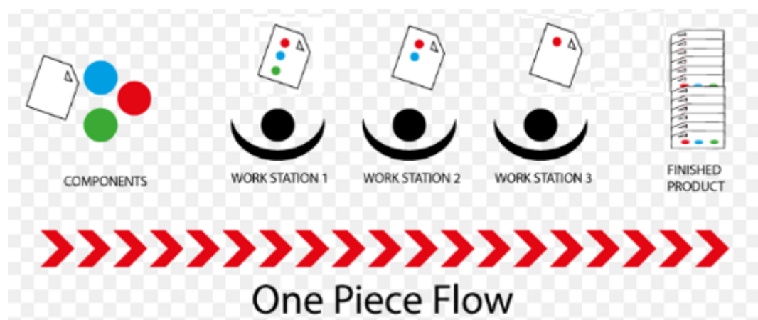
Figure 1: One-piece-flow reduces the work in progress (WIP) level and shortens lead time
