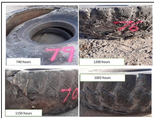
Figure 19: Tyres Failure Modes
