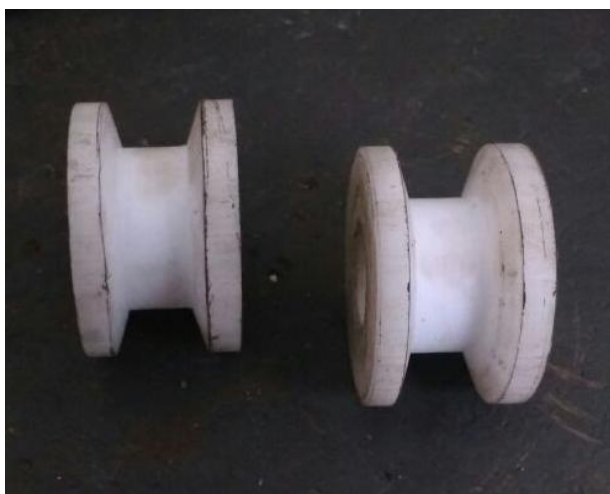
Figure 12: Idler pulleys with a V-groove periphery
