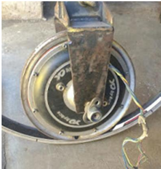
Figure 11: Mating the motor and the rim
