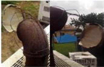
Plate 1: Fabricated apparatus for Method A used to trap emissions from generator
