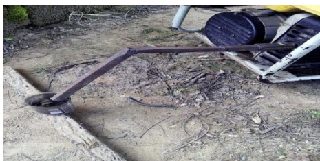
Plate 2: Fabricated apparatus for Method B used to trap emissions from generator
