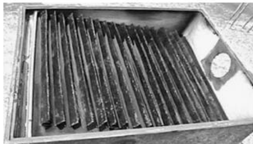
Figure 8: The modified distill with folded, perforated and black coated sheet floating over the water surface (shown with the glass cover removed), P. Valsaraj, 2002, [10]
