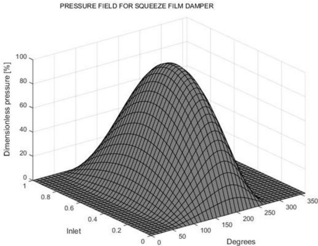
Figure: Final Output of Pressure Field of SFD
