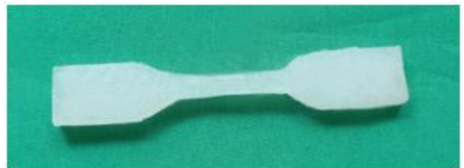
Figure 2: Dumbbell-shaped sample for evaluation of tensile strength
