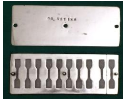
Figure 1: Preparation of samples for evaluation of tensile strength
