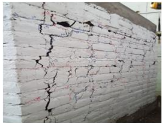
Figure 4: Reinforced adobe wall at the end of the essay
