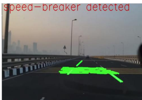
Figure 9: Showing the speed breakers getting detected
