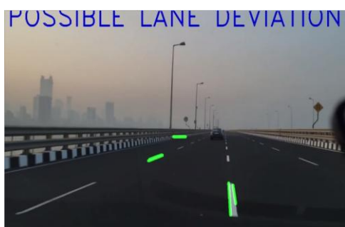
Figure 11: Showing the monitoring of lane-lines
