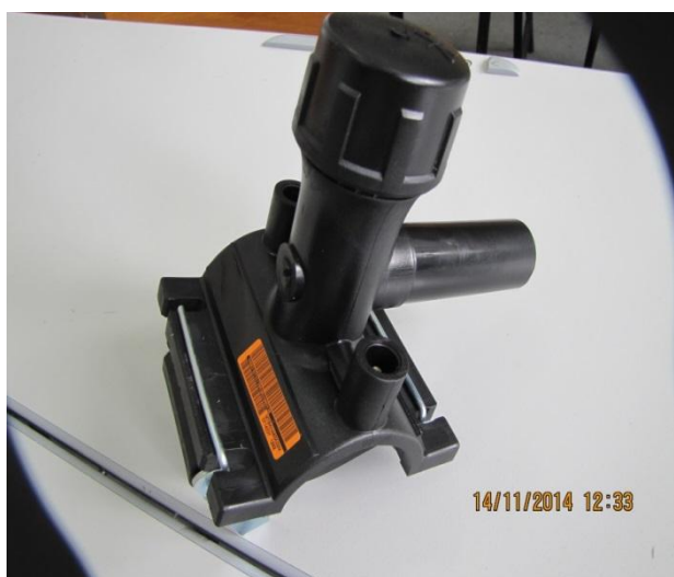
Figure 2: Polyethylene fitting 63-32 mm indiameter before welding
