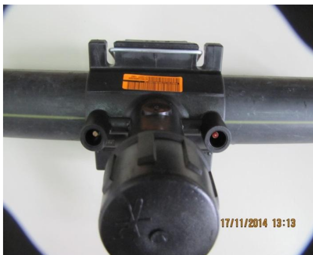
Figure 3: Polyethylene coupler - Dn63-32 pipe assembly resulting from electrofusion welding
