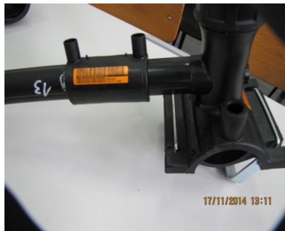
Figure 4: Polyethylene coupler - Dn63-32 pipe assembly resulting from electrofusion welding
