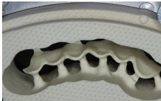
Figure 3: The milling process of the splint
