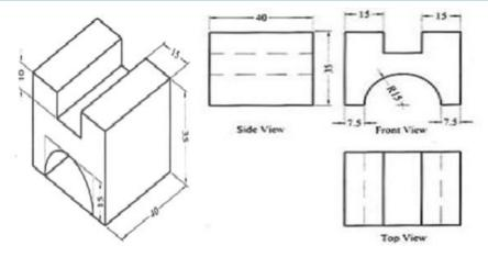
Sectional views: In this object is cut by cutting plane & removing half part of object outside & then view remaining object. i.e.(1) if you draw sectional F.V than always cutting plane is view as a line in T.V& S.V. than based on direction of cutting plane we see the remaining object.(2) Based on direction of cutting plane we see the
