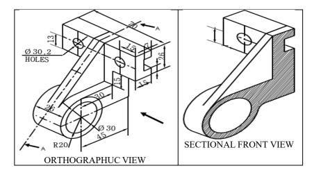
Always after cutting the any object half part of the object removed & than remaining object visualize & make a necessary projection of the object.
