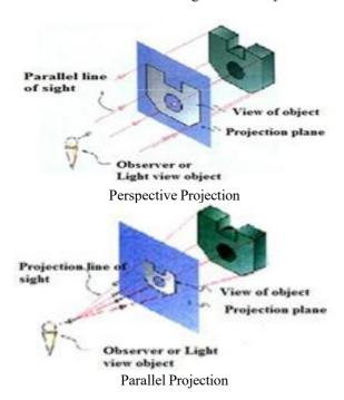
**Drawing steps:** (1) first we **find Area** & draw the **Area** in which we see the F.V & draw that area with Length & Height. [Always we see the Length & Height of any object in F.V.] (2) **Identify the plane** in which we see F.V. [i.e. plane which has some angle between 0° to 180° but not 0° & 180° to eye of observer angle plane is seen as line although it is plane than similarly draw T.V. & S.V.] So firstly, of any 3D object first we must draw
