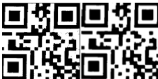
Figure 16: Comparison of QR codes with/without a median filter
