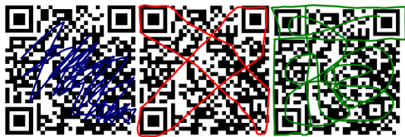
Figure 4: QR code is unable to decode as an essential area has been damaged
