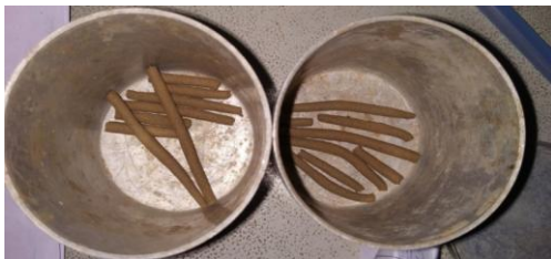
Figure 11: Thread of soil sample for plastic limit test
