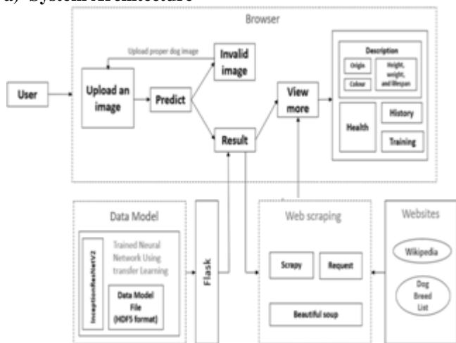
Figure 5: Architecture diagram of the application which show case the front-end and back-end segments
