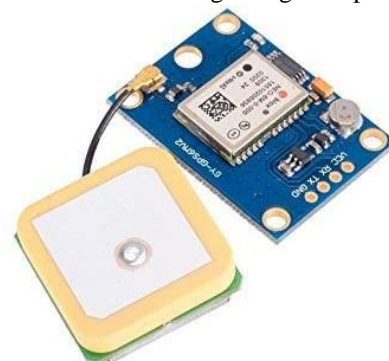
Figure 7: GPS NEO-6 Module used in robotic car
