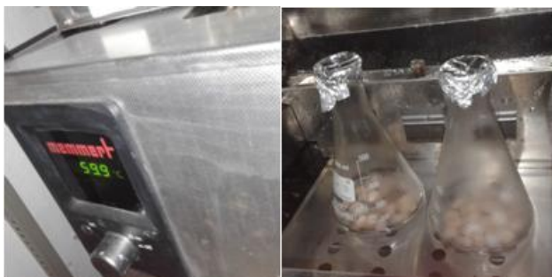
Figure 5: the restored teeth were stored in kcl solution 0.6% and thermal-cycled 45 minutes at 6^\circ\text{C} followed by 45 minutes at 60^\circ\text{C}
