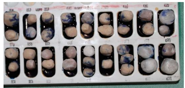
Figure 7 : teeth were immersed in Blue Methylene solution with their apices directed upwards.
